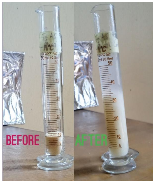
Figure 2: Volume of garri sample in a measuring cylinder before and after swelling.
